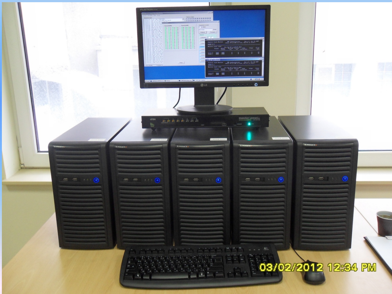
Fig.6. 5 Machine/10 Multimedia DSP Boards/5 x 120 Channels Soft-switch Configuration
